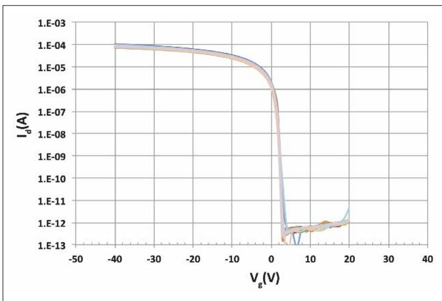
Figure 3: Typical linear transfer curves for SmartKem's *tru-FLEX™* TFTs
